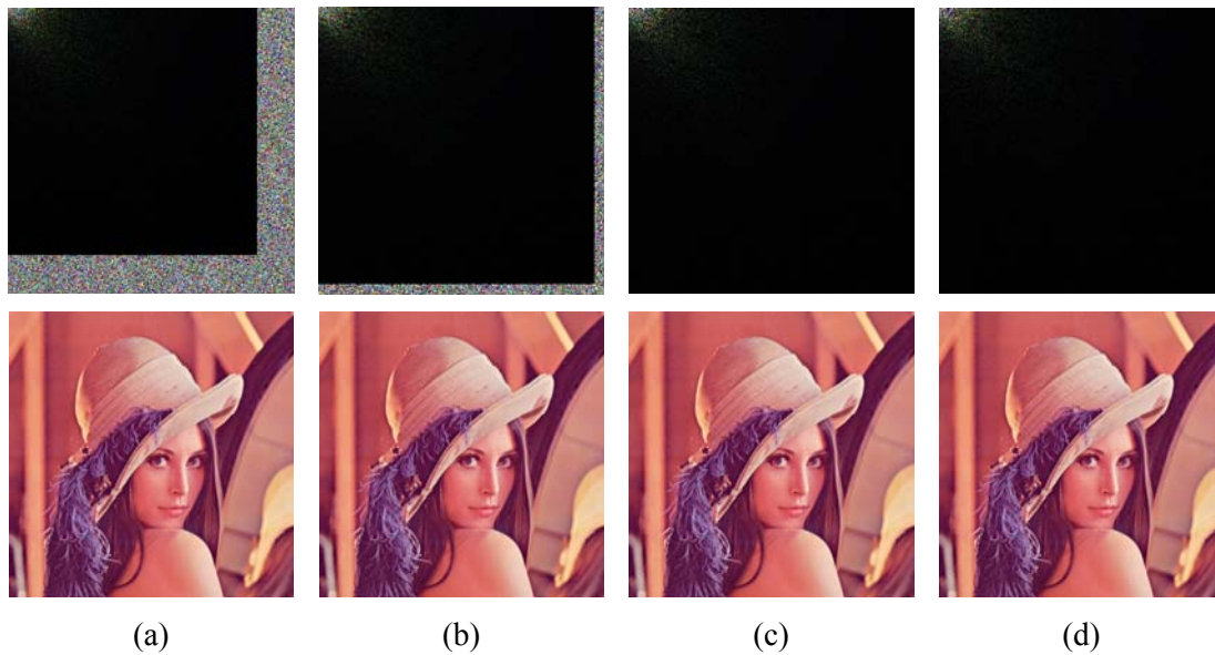
Figure 4.7: Color image encryption by the PRTME_FD algorithm using different recursive sequences. The top row shows the encrypted images. The bottom row shows the reconstructed images. This demonstrates that the PRTME_FD algorithm can encrypt color images and that the original color image is completely reconstructed. (a) P-Fibonacci sequence, p=2 ; (b) P-Lucas sequence, p=2 ; (c) (n, k, p) -Gray code, n=2 , p=0 ; (d) Parametric M-sequence, r=9 , p=2 .
